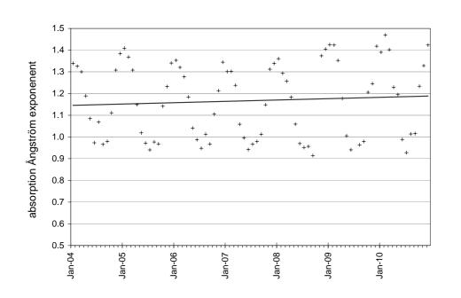
**Fig. 1.** variations in the absorption Ångström exponent at IPR, calculated from the Aethalometer absorption raw data at 7 wavelengths from 370 to 950 nm.
