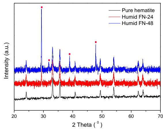
**Fig. 2.** Fig. R2 X-ray diffraction patterns of pure hematite, humid FN-24 and FN-48
