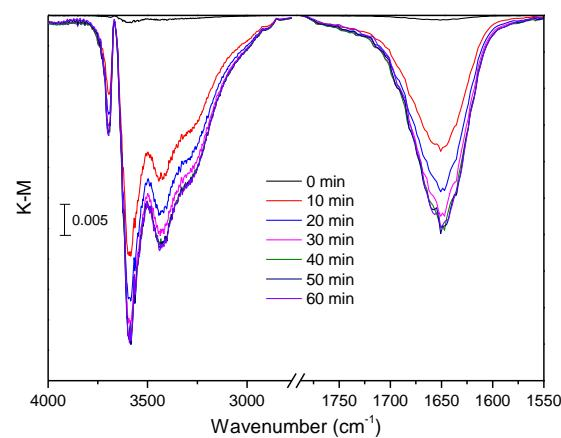
**Fig. 4.** Fig. R4 loss of surface adsorbed water during purge process
