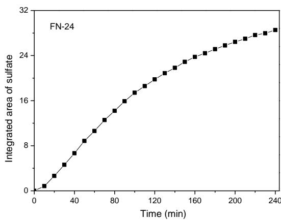
**Fig. 3.** Fig. R3 Time evolution of the integrated areas of sulfate formed on FN-24
