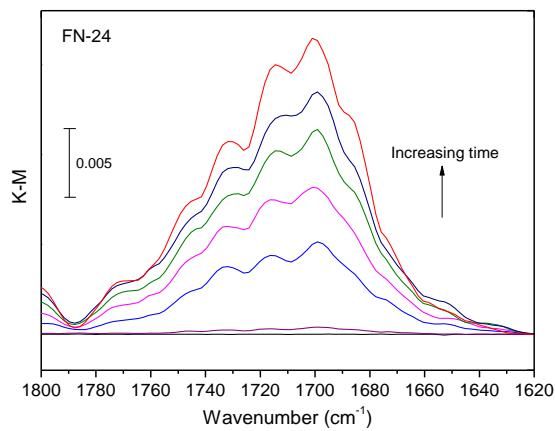
**Fig. 5.** Fig. R5 Adsorption band around 1640 cm⁻¹ after the introduction of gaseous reactant SO₂
