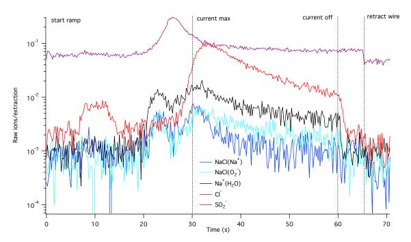
A single sample desorption from May 25, 2011 for unit mass resolution peaks. The main species associated with each nominal mass are indicated. Times when current was applied to the wire are indicated.
