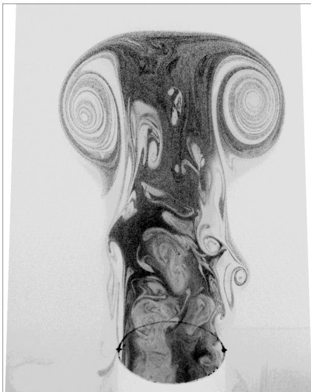
Fig. 1. A cross section of a thermal plume generated in a laboratory with use of a humidifier as a buoyancy source. Distribution of condensed water is shown by gray tone (courtesy : Anna Gorska).
