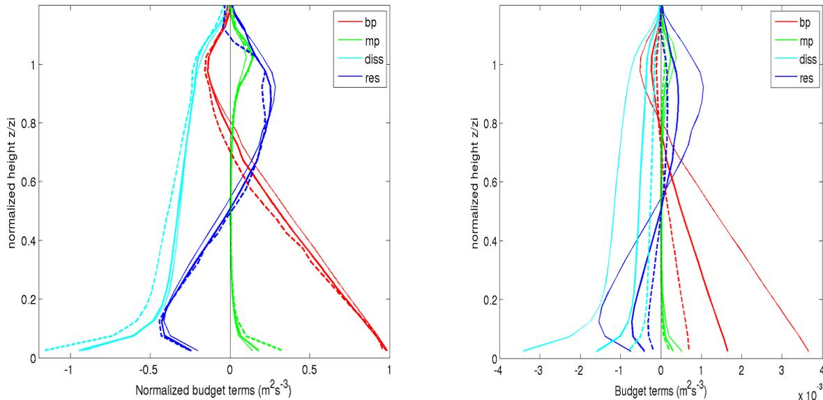
Figure 1: 30-min averaged TKE budget terms normalized (left panel) and not normalized (right panel) at 12:00, 16:00 and 17:00 UTC (thin, thick and dashed lines, respectively). “bp”, “mp”, “diss” and “res” stand for the buoyancy production, the mechanical production, the dissipation and the residual term which should correspond to the transport.
