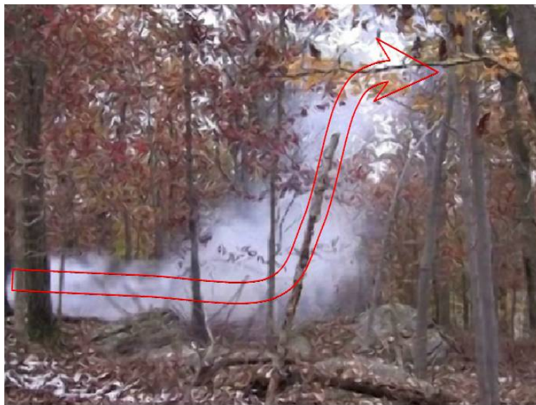
Figure 3 Updraft motion detected in forest canopy in the early morning by smoke experiment.
