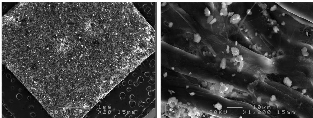
Suppl. Fig. 1. SEM images of dust particles collected on cellulose filter (2009 dust).
