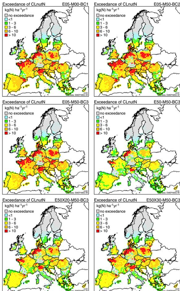
**Fig. 12.** Exceedances of the critical loads for nutrient nitrogen (CL<sub>nut</sub>(N)) in the EU28<sup>+</sup> region, EMEP MSC-W model, for the six scenarios.
