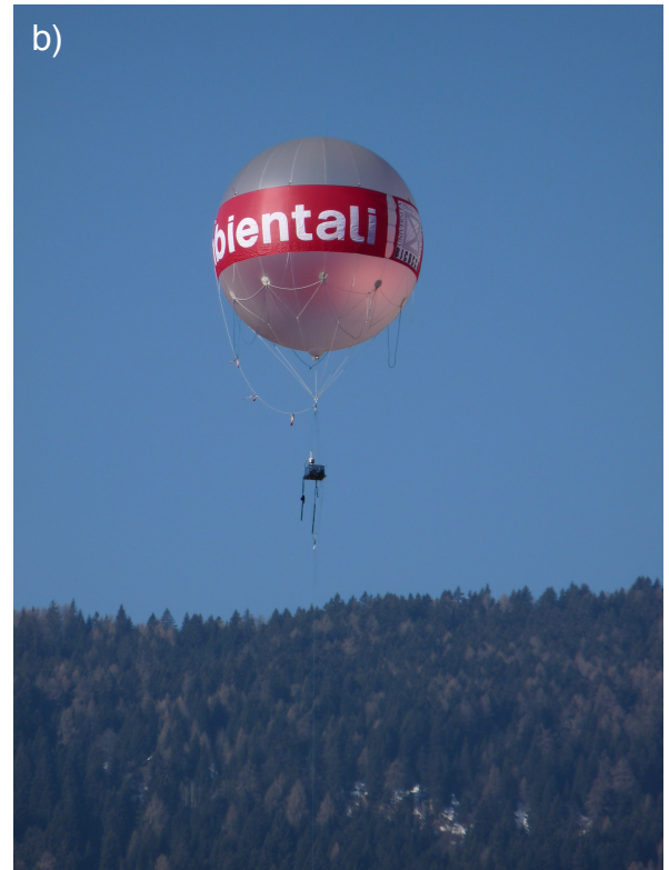
Figure 1. a) Location of the three sampling sites: Terni in Central Italy (Terni Valley), Milano in Northern Italy (Po Valley) and Merano in the Alpine region (between Passiria and Val Venosta Valleys); b) The tethered balloon flying over Merano with the instrumentation package.
