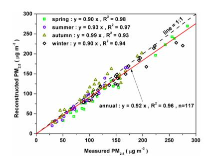
**Fig. 4.** Correlation between reconstructed and measured  $PM_{2.5}$  mass concentrations in four seasons. Also shown are the linear regression lines with regression equations.
