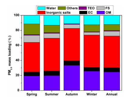
**Fig. 5.** Chemical mass closures of  $PM_{2.5}$  mass concentrations in four seasons. The major chemical components include inorganic salts, organic matter (OM), elemental carbon (EC), fine soil (FS), trace element oxides (TEO), water content, as well as others that were unidentified.
