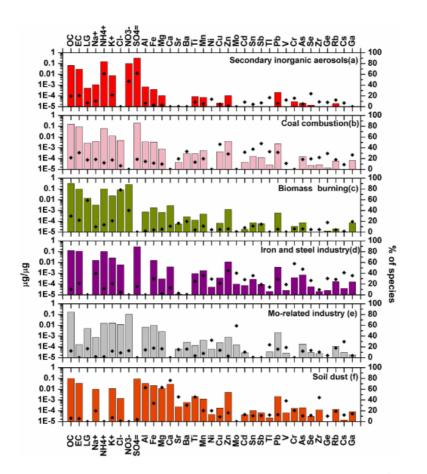
**Fig. 6.** Six source profiles (bars) resolved from the PMF model (in unit  $\mu g \mu g^{-1}$ ). Also shown is contribution percentages (black dots) from each source factor (in unit %).
