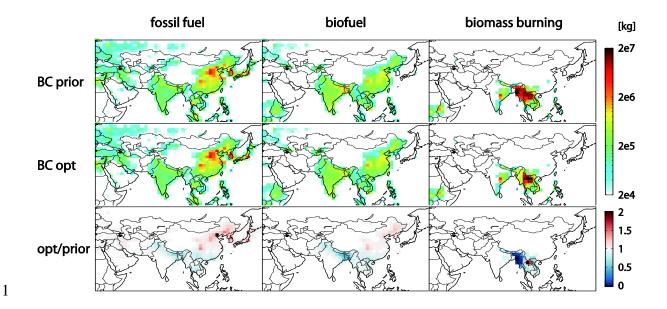
Figure 3 BC emissions from different sources during 1 March–1 April 2010. The top row shows the prior inventory, the middle row shows the posterior inventory, and the bottom row shows the scaling factors.
