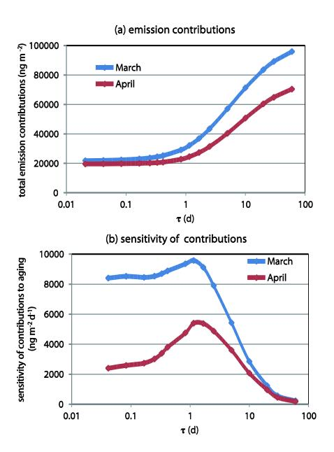
Figure 8 Effect of BC aging on transpacific transport of BC. (a) Total emission contributions to BC over the North Pacific observational domain as a function of BC aging rate. (b) Sensitivity of total BC transported to the observational domain from all the sources to the rate of BC aging (i.e., the rate of change of emissions contributions in (a) with respect to the e-folding aging time  $\tau$ ).
