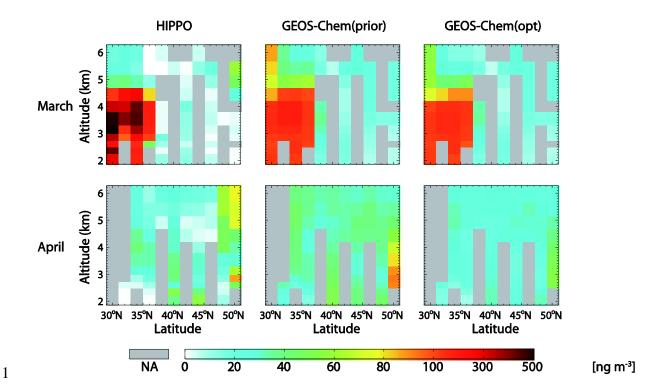
Figure 2 BC vertical profiles in the observational domain (150–160 W) on 29 March 2010 (top) and 13 April 2010 (bottom). HIPPO aircraft observations (left) and GEOS-Chem model estimates (sampled along aircraft track) using the prior (center) and the optimized (right) BC emissions are shown.
