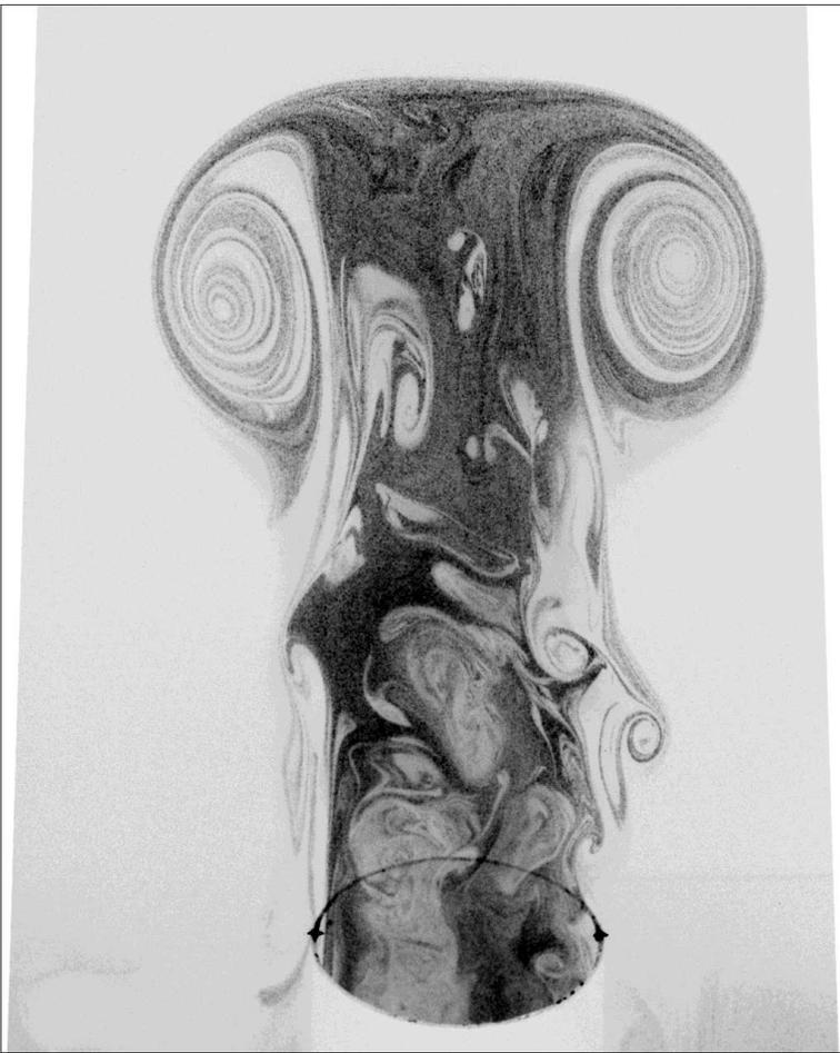
**Fig. 5.** A cross section of a thermal plume generated in a laboratory with use of a humidifier as a buoyancy source. Distribution of condensed water is shown by gray tone (courtesy : Anna Gorska and Szymon Malinowski).
