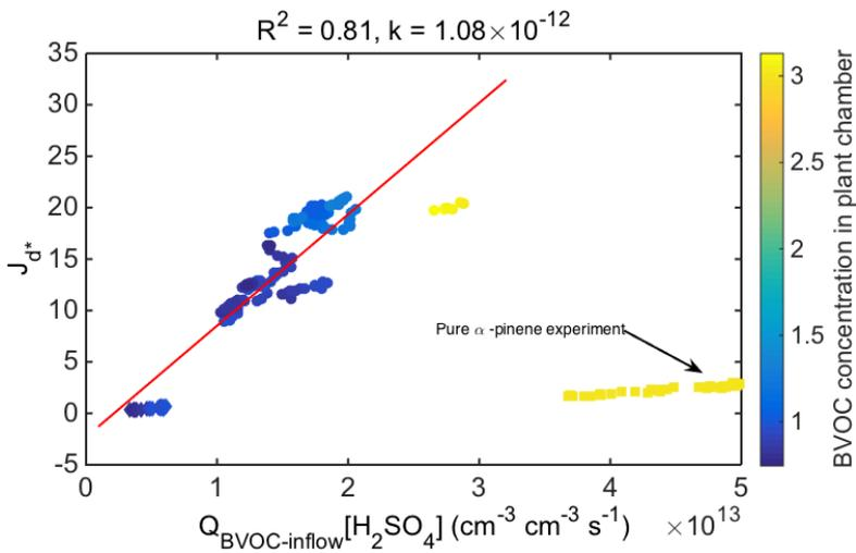
**Figure 5.** Particle formation rates ( $J$ ) as function of the product of BVOC inflow and sulphuric acid concentration. Marker colours indicate the corresponding monoterpene concentration from the inlet flow of JPAC reaction chamber. The pure  $\alpha$ -pinene experiments indicated in the figure were not included in the linear fit.
