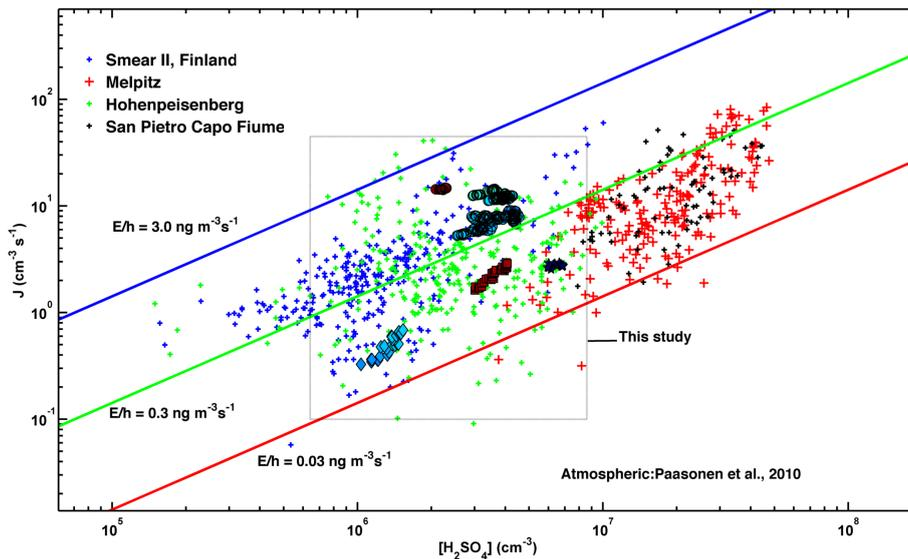
**Figure 8.** Comparison of our results to atmospheric formation rate studies as reported in Paasonen et al. (2010). Nucleation parameterizations of the form  $J = K_E \cdot E/h \cdot [\text{H}_2\text{SO}_4]$ , with  $K_E = 4.5 \times 10^{-6} \text{ m}^3 \text{ ng}^{-1}$  and three different source rates  $E/h$  are shown together with measured data points.
