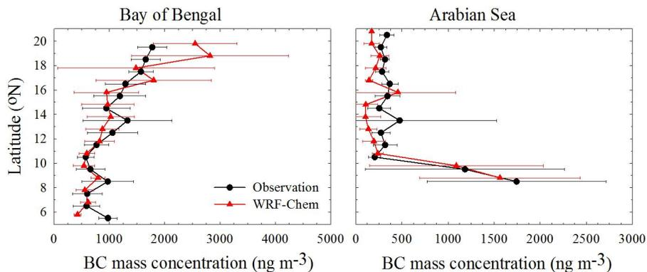
**Figure 4.** WRF-Chem predicted and observed latitudinal gradients in BC mass concentrations along the ICARB ship-track in the Bay of Bengal and Arabian Sea regions. Horizontal bars represents one sigma (SD) variation in BC mass concentration averaged over a 1° latitude bin.
