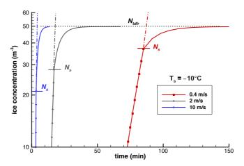
Figure 1. Time evolution of ice particle concentration in a parcel of air undergoing lifting at three different updraft velocities. Cloud base is at 700 mb and +2°C. Lifting stops at -10°C and the parcel remains at that level. The TDFR model is initialized with an INP concentration given by Eq. (3). The horizontal line segments at  $N_s$  indicate the ice concentrations when the lifting stops.  $N_{tdfr}$  is the asymptotical value of ice concentration while the parcel is at -10°C.
