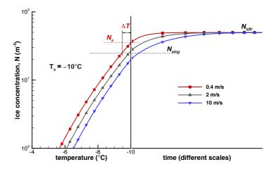
Figure 2. The same data as in Fig. 1 displayed as a function of temperature during the lifting of the parcel and as a function of time after that. Time scales differ for the three cases.  $N_s$  and  $\Delta T$  are indicated for 0.4 m s<sup>-1</sup> updraft velocity.  $\Delta T$  is defined in Eq. (5) with w = 0.15 °C min<sup>-1</sup> for this case.  $N_{sing}$  is the ice concentration from Eq. (3) for - 10°C using the singular approximation.
