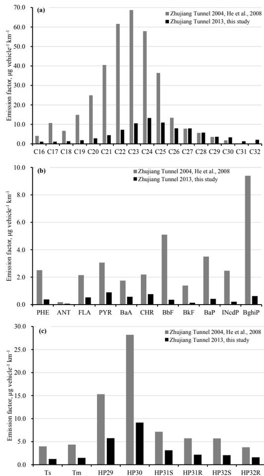
**Figure 4.** Comparison of organic compounds emissions in the Zhujiang Tunnel sampling in 2004 and 2013.
