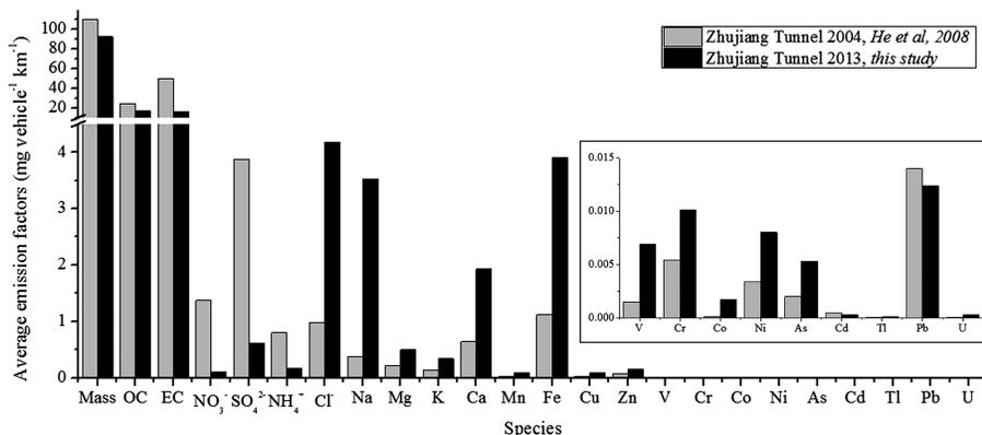
**Figure 3.** Comparison of PM<sub>2.5</sub>, OC, EC, WSII and metal emissions in the Zhujiang Tunnel sampling in 2004 and 2013.
