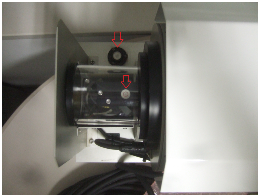
Fig. 2. Two horizontal levels embedded in the base plate (upper arrow) and in a plate holding the reflecting mirror (lower arrow) were used to adjust the zero angle of the reflecting mirror.
