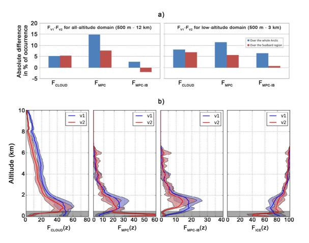
Figure 4. a) Absolute differences in % of occurrence between occurrences computed from V1 and V2 DARDAR products for total cloud, MPC and MPC-IB and b) Mean vertical profiles of clouds, MPC, MPC-IB and ice clouds occurrences computed from V1 (blue lines) and V2 (red lines) DARDAR products for April 2007 over the Svalbard region. Filled areas represent the standard deviation.
