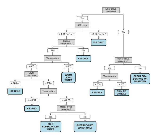
3 Figure 1. Representation of the DARDAR algorithm retrieval steps for cloud thermodynamic phase.
