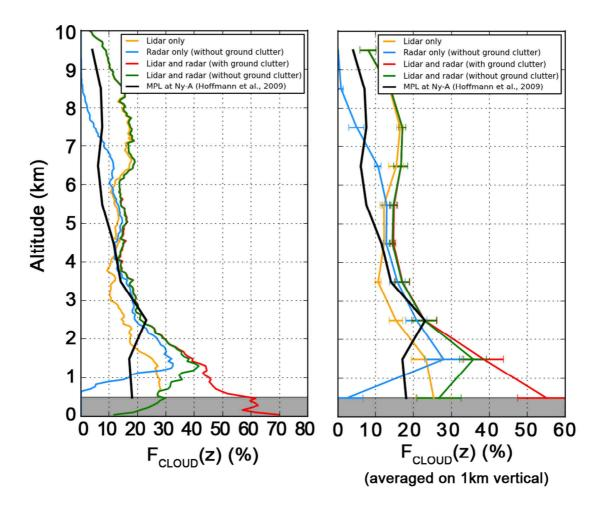
Figure 2. Vertical profiles of cloud occurrences over the Ny-Alesund station during March and April 2007. The black line refers to ground based lidar observations at 1 km vertical resolution (Hoffmann et al., 2009) and coloured lines refer to a DARDAR product according to different configurations and settings. DARDAR retrievals have a vertical resolution of 6 0m on the left panel and 1 km on the right panel.
