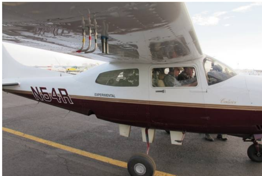
Figure 2. Photograph of the Cessna 210 aircraft that sampled over the Uinta Basin in February 2013. Three inlets and two temperature and humidity probes were installed under the starboard wing.
