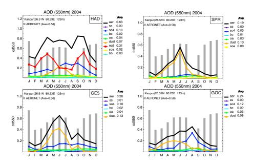
**Figure 6.** AOD of total aerosol (aer) and components (ss,  $so_4$ , bc, oa, dust,  $no_3$ , soa and bb) at Kanpur for 2004 in 4 models, HAD (upper left), SPR (upper right), GES (lower left) and GOC (lower right). The gray bar represents measurement from AERONET. The annual mean AOD is followed after the name of each symbol. NOTE: bc and oa represent emission from fossil fuel only and bb represents emission from biomass burning only).
