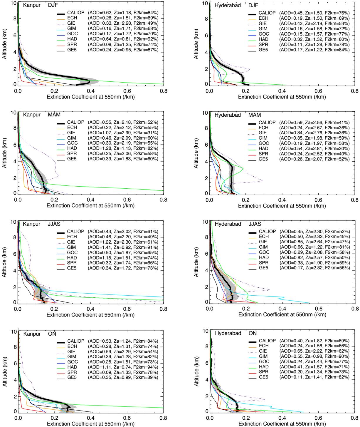
Figure 8. The seasonal mean of vertical profile of extinction coefficient (units: 1/km) at (a) Kanpur, and (b) Hyderabad from CALIOP and seven models. Units of Za is km. The corresponding averaged AOD, Za and F<sub>2km</sub> are listed after each symbol name. The gray shaded area in CALIOP shows one standard deviation relative to 2006-2011 averages.
