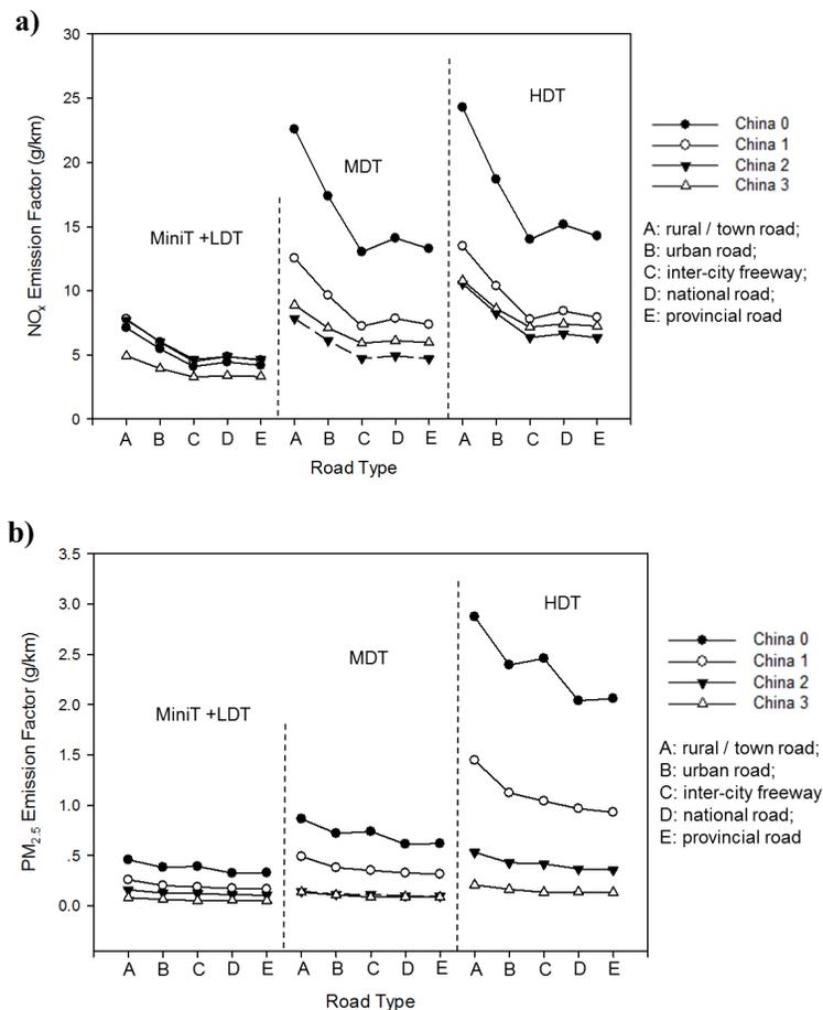
**Figure 6.** Emission factors on different roads **(a)**  $\text{NO}_x$  emission factors; **(b)**  $\text{PM}_{2.5}$  emission factors.
