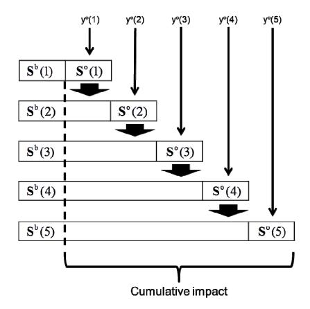
Figure 2. Schematic diagram of calculating cumulative impact in CarbonTraker.  $S^b(\bullet)$  indicates the analysis sensitivity to background at each analysis cycle within five weeks of lag, where  $\bullet$  denotes each week from 1 to 5.  $S^o(\bullet)$  indicates the analysis sensitivity to observation at each analysis cycle.
