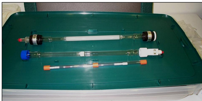
Fig. 6: The hollow quartz denuder from URG Corporation (middle).
