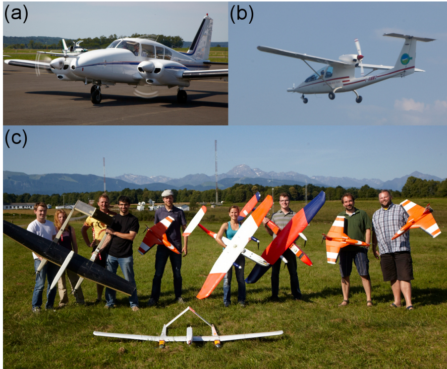
Fig. 5. (Top left) The SAFIRE Piper Aztec aircraft, (top right) the CNR Sky Arrow aircraft, and (bottom) the RPAS teams participating during most of the BLLAST campaign. The RPAS presented from left to right are: MASC (University of Tübingen, Germany), SUMO (University of Bergen, Norway), M2AV (2 planes, Technical University Braunschweig, Germany), SUMO (2 planes), and one MASC in front.
