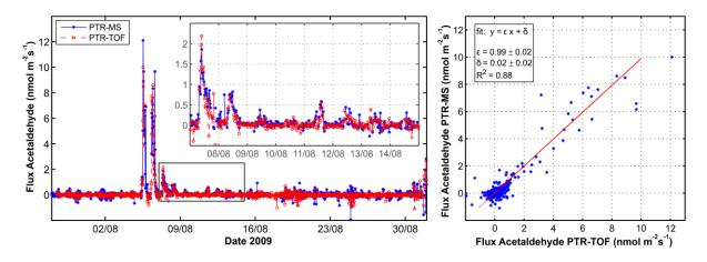
**Figure S1**. Comparison between acetaldehyde fluxes measured by PTR-TOF and fluxes measured by the PTR-MS (on m/z 45) for a time period from 28 July until 1 September 2009 together with a scatter plot specifying the regression parameters for a linear regression between both data sets ( $F_{PTR-MS}=0.99*F_{PTR-TOF}+0.02$ ,  $R^2=0.88$ ).
