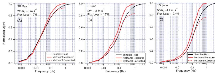
**Fig. 7.** Ogives of sensible heat and methanol (before and after attenuation correction) for three days of different wind speeds and atmospheric stability. Flux loss at high frequencies increased with wind speed and stability, where a greater contribution to the flux came from smaller eddies.
