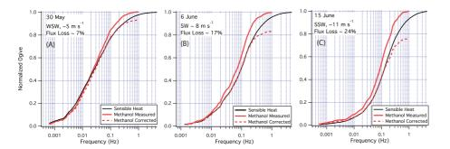
**Fig. 7.** Ogives of sensible heat and methanol (before and after attenuation correction) for three days of different wind speeds and atmospheric stability. Flux loss at high frequencies increased with wind speed and stability, where a greater contribution to the flux came from smaller eddies.
