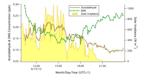
**Fig. 4.** Concentrations of acetaldehyde and DMS on 15 June, along with solar irradiance. With strong winds from SSW (over the Plymouth Sound), DMS concentration was detectable by the PTR-MS and demonstrated the expected diel variability, while acetaldehyde concentration peaked in solar noon and declined for the rest of the daytime.
