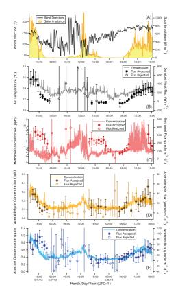
**Fig. 9.** As with Fig. 8, but for  $6 \sim 8$  June. During this windy period, acetaldehyde and acetone fluxes as well as concentrations were higher during the day, following the trend of heat flux. Acceptable flux measurements could not be made for most of 7 June and a few hours on 8 June due to corruption of the sonic anemometer data in the presence of heavy rain.
