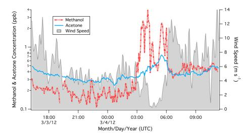
**Fig. 3.** Concentrations of methanol and acetone during 3 ~ 4 March, along with wind speed (from SW). Greater fluctuations were apparent in the concentration of methanol than in acetone on short timescales, in part due to greater spatial heterogeneity of methanol sources. Methanol concentration increased by an order of magnitude when the wind ceased, likely due to a shallow nocturnal boundary layer.
