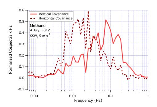
**Fig. 14.** Normalized methanol cospectra for vertical covariance (same as Fig. 5) and horizontal covariance on 4 July. The horizontal cospectrum peaked at a lower frequency than the vertical cospectrum, likely related to spatial inhomogeneity.
