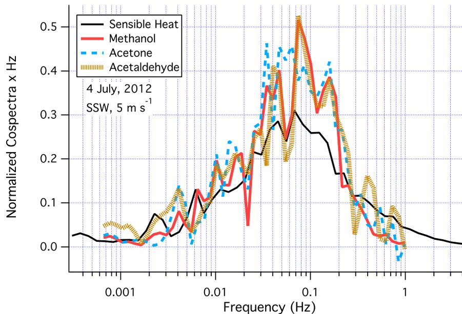
**Fig. 5.** Cospectra of sensible heat, methanol, acetone, and acetaldehyde normalized to the respective fluxes during 4 h of steady winds on 4 July. Trimming of plants immediately upwind resulted in exceptionally large fluxes and well-defined cospectra for all three OVOC species, which showed good agreement with each other.
