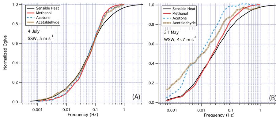
**Fig. 6.** Ogive of sensible heat, methanol, acetone, and acetaldehyde normalized to the respective fluxes for 4 July **(A)** and 31 May **(B)**. On 4 July (same period as Fig. 5), the ogives of different OVOCs demonstrated good agreement with each other and to that of sensible heat due to strong local emissions and steady winds. In contrast, rising winds on 31 May caused increasing concentrations of acetone and acetaldehyde, which is evident in the greater ogives at low frequencies.
