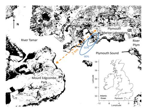
**Fig. 1.** Map of the Plymouth Sound and the location of Plymouth. The small and large ellipses illustrate the approximated 60 % and 90 % (cumulative) flux footprint under typical conditions. At ~ 2 km SW of the PLM and separated by the River Tamar, the forested Mount Edgcombe Park likely lies outside of the flux footprint.
