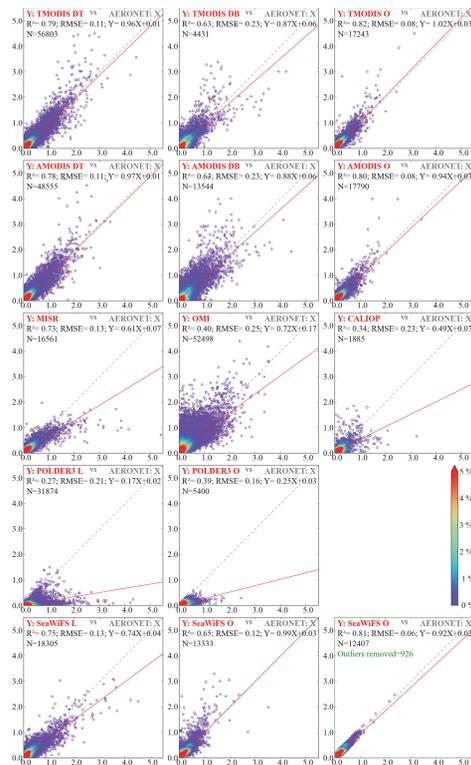
**Fig. 6.** Regression fits of AERONET AOD (x-axes) to AOD measured by spaceborne sensors (y-axes). Satellite data were pre-screened by QA as explained in Sect. 4. The color of each data point indicates the percentage of all data points on the plot that fall within 0.05 AOD of this point (in Cartesian coordinates). Scatter plot in the green frame demonstrates the results of the possible data outlier detection and removal procedure described in Sect. 5.
