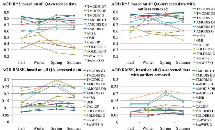
**Fig. 10.** Seasonal dependence of squared linear fit correlation coefficient ( $R^2$ ) and root mean square error (RMSE) statistics between the collocated spaceborne and ground-based (AERONET) observations of AOD, based on the data in Table 3.
