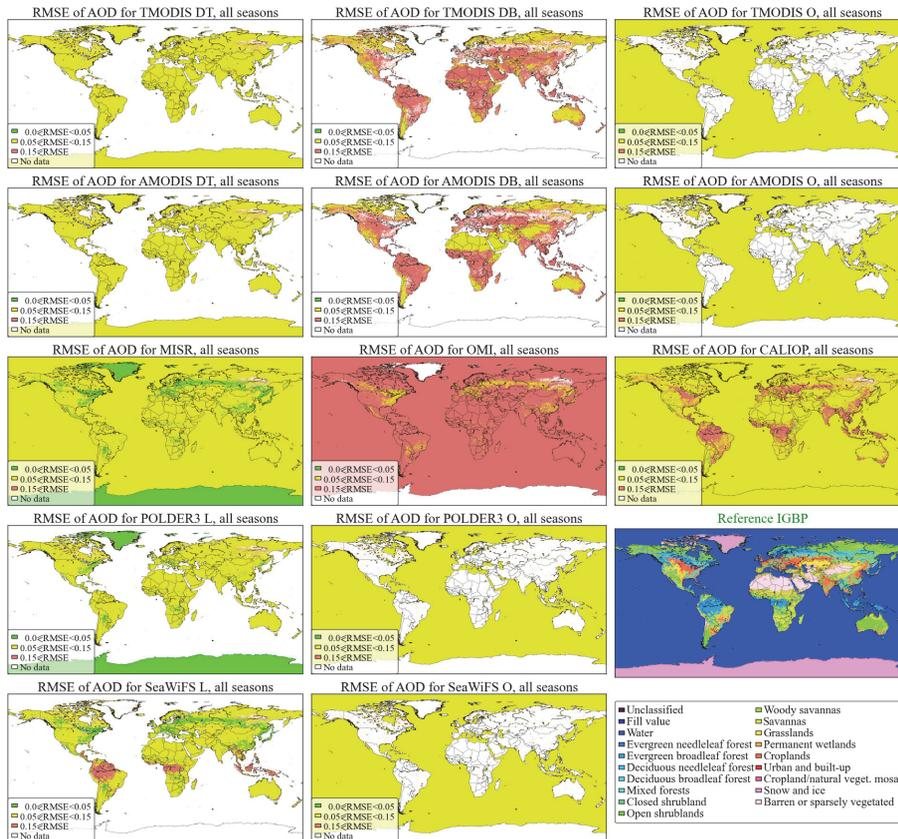
**Fig. 14.** Land cover type dependence of root mean square error (RMSE) between the collocated spaceborne and ground-based (AERONET) observations of AOD. Areas corresponding to each IGBP land cover type (bottom right inset) are colored based on the average of the data from those AERONET sites that reside in these areas. The statistics were calculated based on the data that were pre-filtered by QA and screened of outliers as described in Sects. 4 and 5.
