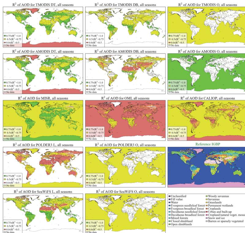
**Fig. 13.** Land cover type dependence of squared linear fit correlation coefficient ( $R^2$ ) between the collocated spaceborne and ground-based (AERONET) observations of AOD. Areas corresponding to each IGBP land cover type (bottom right inset) are colored based on the average of the data from those AERONET sites that reside in these areas. The statistics were calculated based on data that were pre-filtered by QA and screened of outliers as described in Sects. 4 and 5.
