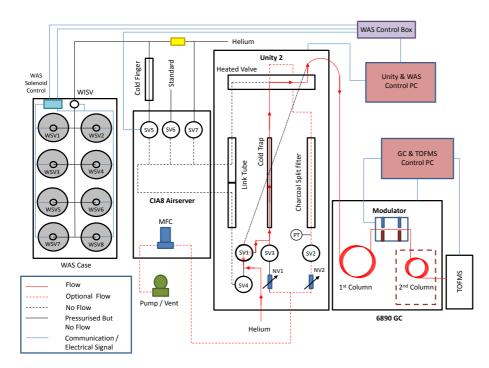
**Fig. 1.** Schematic of the finalised TD-GC  $\times$  GC-TOFMS sampling set-up. SV = solenoid valve. NV = Needle valve. MFC = Mass flow controller. WISV = WAS inlet solenoid valve. WSV = WAS solenoid valve. PT = Pressure transducer.
