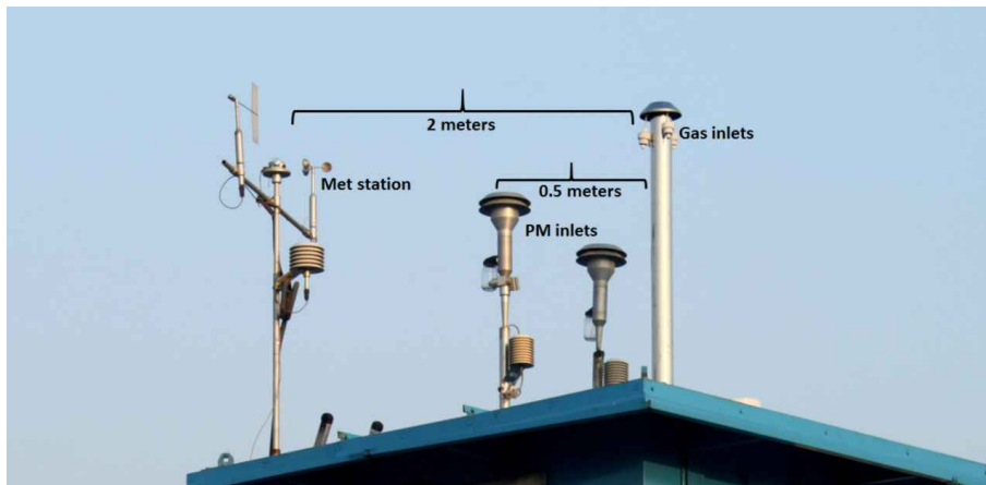
Fig. 5. Picture of the co-located instrument inlets and meteorological sensors ( \sim 20 m.a.g.l.) at the IISER Mohali atmospheric chemistry facility.
