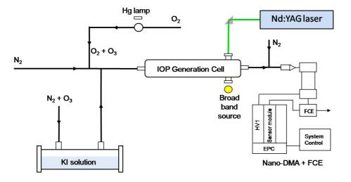
**Fig. 1.** Experimental setup showing the two different types of light sources (W/Xe lamp or Nd:YAG laser) used to photolyse and distinguish between  $I_2$  and HOI.
