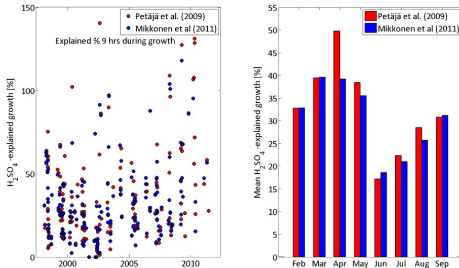
**Fig. 12.** The timeseries of the percentage which H<sub>2</sub>SO<sub>4</sub> explains of the growth **(A)**, its yearly variation **(B)**. Months with less than 5 cases where the percentage has been calculated have been discarded.
