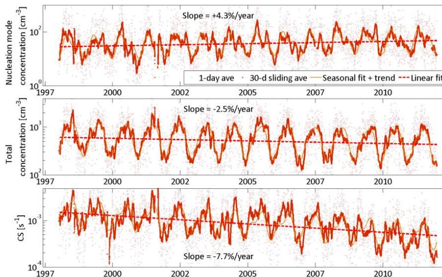
**Fig. 8.** Trends in nucleation mode and total concentration as well as condensation sink 1998–2011. The light red dots are 1 day averages, the solid dark red line is the 30 d sliding average, the thin orange line is the sinusoidal seasonal fit with the linear trend added and the red dashed lines are the linear fits.
