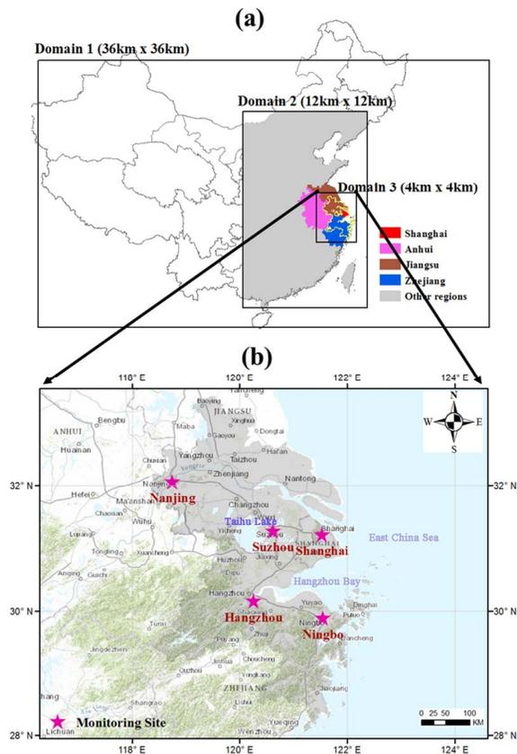
**Fig. 1.** Model domain and location of measurement sites. **(a)** Three nested domain grids for WRF/CMAQ modeling. **(b)** Location of field monitoring sites. The yellow border in **(a)** and gray area in **(b)** constitute the YRD region. The five regions indicated by different colors in panel **(a)** were used for WRF/CMAQ sensitivity analyses, with biomass burning emissions set to zero in each region to determine their effects on concentrations of  $PM_{2.5}$  and carbon species.
