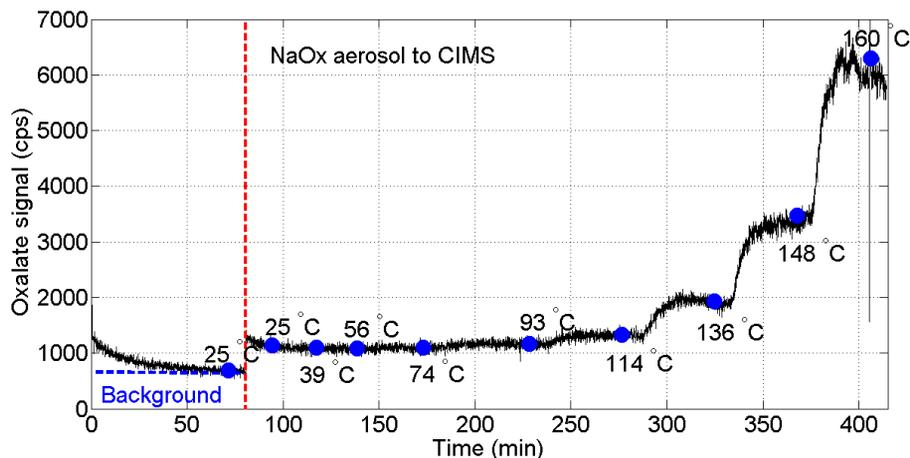
**Fig. 4.** Volatility of NaOx aerosol with TPD Aerosol-CIMS (NaOx (1)). The detected oxalate signal when aerosol was heated stepwise from room temperature to 160°C as a function of time (minutes from the beginning of the experiment) is illustrated in the figure (black solid line). Also the average oxalate signal at different temperatures is plotted (blue dots). The average background oxalate signal was subtracted from the oxalate signal for further analysis.
