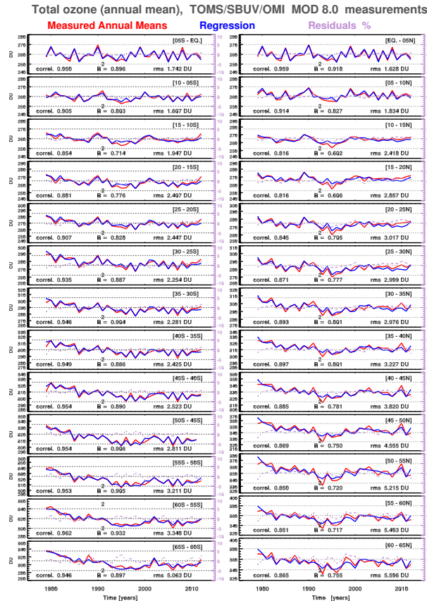
Fig. 5. Observed TOMS/SBUV/OMI V8.0 (red) annual zonal mean total ozone columns for 5° wide latitude bands from 65° S to 65° N and regressed (blue) ozone obtained from regression models (with winter mean EHF dynamical proxy). The right hand scale in each panel gives the residuals in percent (violet). The correlation, R^2 and rms are also noted for each latitude band.
