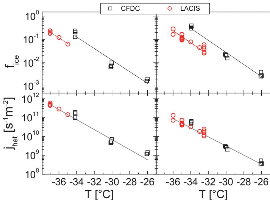
**Fig. 2.** Measured  $f_{ice}$  and derived  $j_{het}$  for CFDC and LACIS for two particle types (left panels: 300 nm Fluka kaolinite coated with LG at 80 °C; right panels: 700 nm Fluka kaolinite (no coating)).
