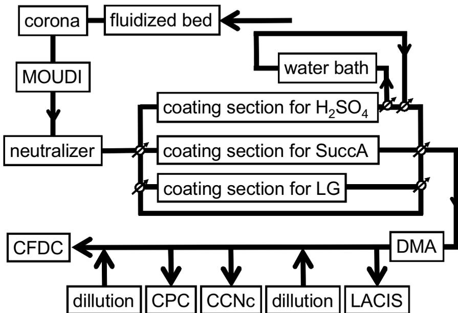
Fig. 1. Set-up of the particle generation.
