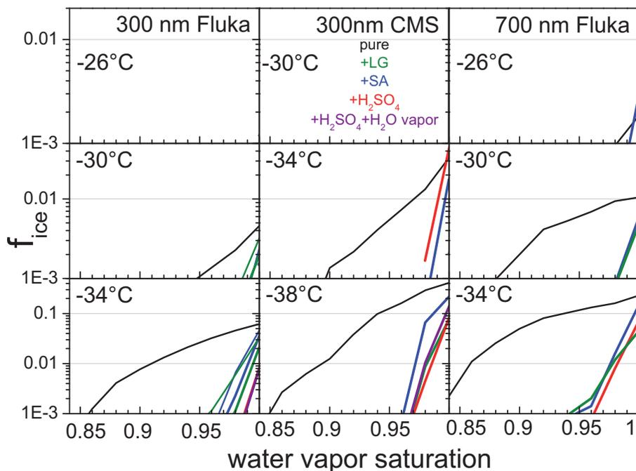
**Fig. 5.**  $f_{ice}$  measured with the CFDC for  $S_w < 1$ . Thinner lines indicate medium thick coatings, thicker lines represent thick coatings. The type of coating is indicated by colors, the color coding can be seen in the upper middle panel.
