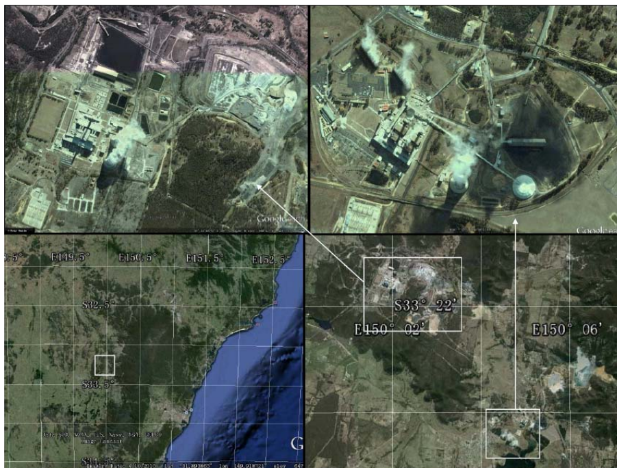
Fig. 4. An aerial view of two coal power plants that were found at the location of the origin of the pollution track ( 33.38^{\circ} S, 150.05^{\circ} E) that is shown in Fig. 3. The power plants are 7 km apart from each other.
