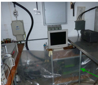
Fig. 2. Setup of the laser spectrometer at the Büel measurement site of the research catchment Rietholzbach. (a) Inlet of the sampling system. (b) Setup of the Picarro L1115-i cavity ring-down laser spectrometer in the cellar of the measurement field. (c) Flow diagram of the setup including the inlet and the laser spectroscopic measurement system.
