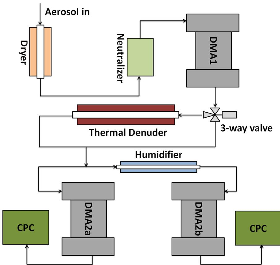
Fig. 1. A schematic of the VH-TDMA instrument system.
