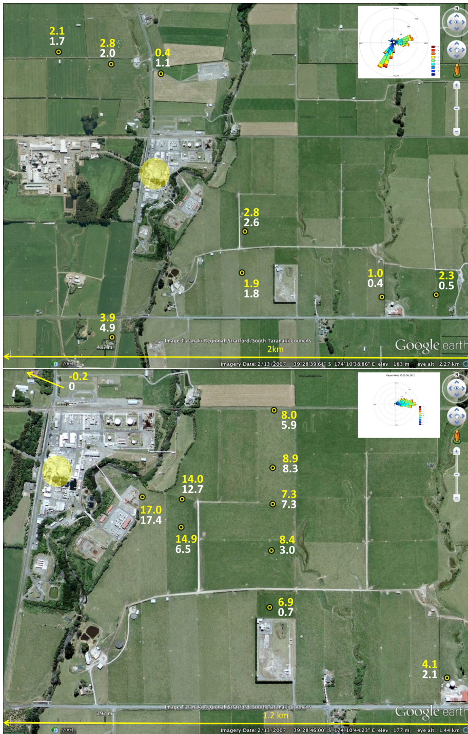
Figure 6. CO 2 ff in grass samples collected on August 14 th , 2012 (top) and October 24 th , 2012 (bottom). The observed CO 2 ff derived from \Delta^{14}\text{C} is shown in yellow, and the modeled CO 2 ff prediction is shown in white. Markers indicate the exact sampling location. A wind rose showing the direction of the wind patterns over the previous one week period is inset (bars indicate the direction the wind is traveling to). In the lower panel the point indicated with the arrow was measured 500 m to the north-west, off the map.
