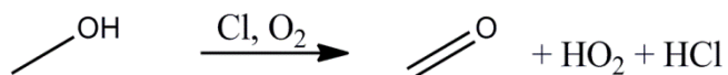
Figure S-2. Methanol oxidation mechanism by atomic chlorine added to the model reactions.
