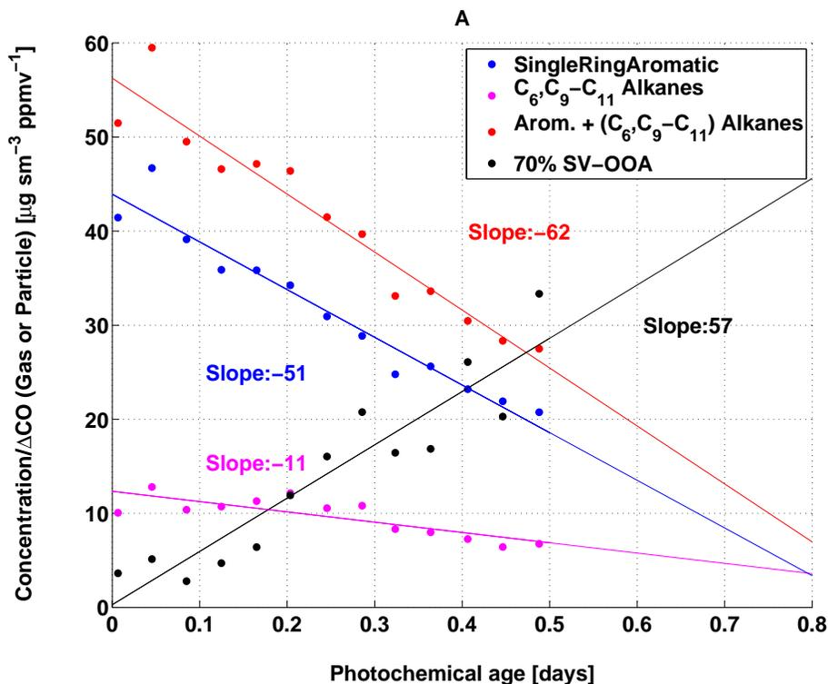
**Fig. 4.** Measured PMF OOA factor concentrations normalized by CO enhancement ( $\Delta\text{CO}$  is the ambient CO minus the estimated background CO (105 ppb)) as functions of photochemical age. Also shown are lumped gas-phase VOC concentrations normalized by  $\Delta\text{CO}$ . See Table 6 for the chemical speciation of each lumped species.
