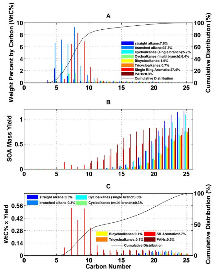
**Fig. 2.** Distribution of mass by chemical class based on California fuel-sale data comprising 13% diesel and 87% gasoline, by volume (top panel). Distribution of compound specific SOA mass yields (middle panel). Relative contributions of each group of species to predicted SOA, calculated as the yields multiplied by weight percent (by carbon) in liquid fuel (bottom panel). Data are from Tables S5, S6, and S8 of Gentner et al. (2012).
