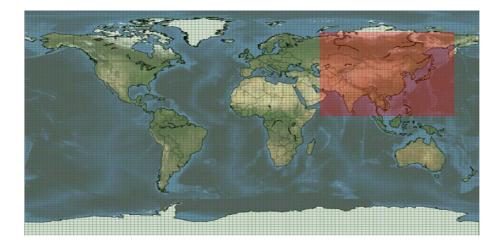
**Fig. 1.** TM5 global grid  $(3 \times 2)$  with zoom over Asia  $(1 \times 1)$ .
