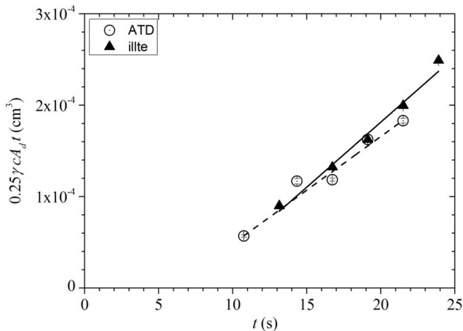
**Fig. 5.** Plot of  $0.25\gamma_{exp}\bar{c}N_dA_d t$ , versus the contact time ( $t$ ) for  $N_2O_5$  with dust aerosols in the AFT. The lines are least-squares fits to the illite (solid line) and ATD (dashed line) datasets. The error bars are statistical ( $2\sigma$ ) only.
