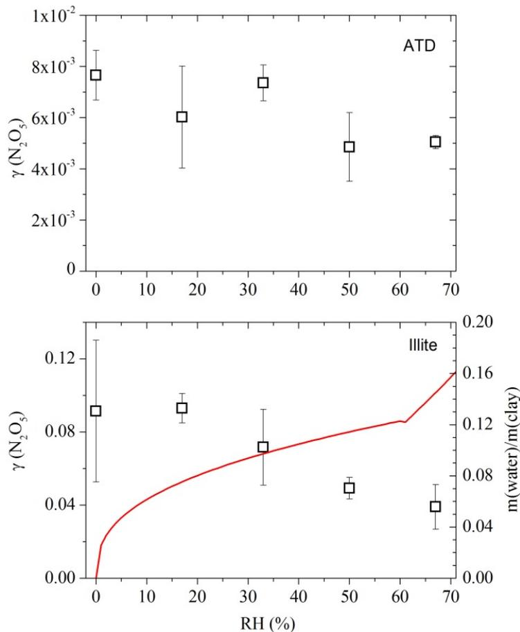
**Fig. 6.** Uptake coefficients of  $\text{N}_2\text{O}_5$  at different relative humidities to illite and ATD. The ratio of the mass of absorbed water to that of dry illite (lower panel, red curve, right y axis) is also plotted as a function of RH (Hatch et al., 2012).
