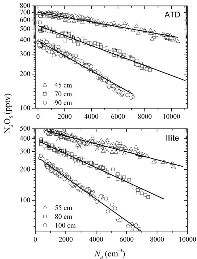
**Fig. 4.** Exponential dependence of the measured  $N_2O_5$  mixing ratio on the dust aerosol number concentration at three different injector positions at  $RH = 0\%$ .
