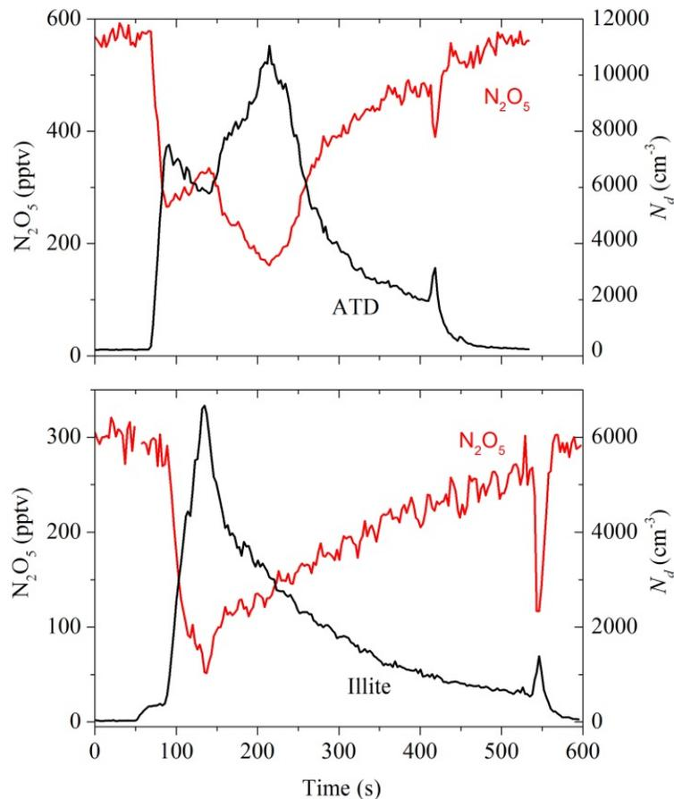
**Fig. 3.** Response of the  $N_2O_5$  mixing ratio (left axis) to the introduction of mineral dust aerosols (right y axis) into the flow tube at  $RH = 0\%$  when the injector was at 70 cm. The time between acquisition of neighbouring data points is  $\sim 3$  s.
