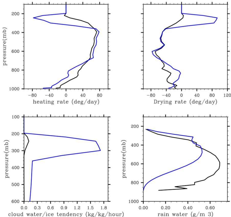
**Fig. 4.** Vertical profiles of heating, drying, cloud water and ice tendencies, and rain water distribution for clean (black) and polluted (blue) conditions.
