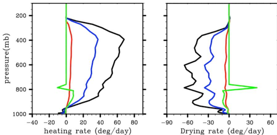
**Fig. 3.** Heating rate (left), and drying rate (right), for grid resolution of 30 km (black), 10 km (blue), 3 km (red) and 1 km (green).
