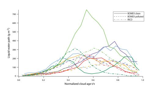
**Fig. 10.** Time series of liquid water path. Liquid water path is the cloud-integrated LWC divided by maximum cross-sectional area.
