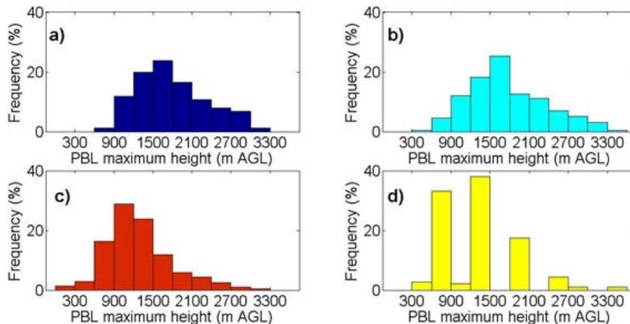
**Fig. 6.** Histograms for measured and modelled PBL top daily maximum heights during 2010, (a) Polly<sup>XT</sup>, (b) ECMWF, (c) TAPM and (d) SAWS.
