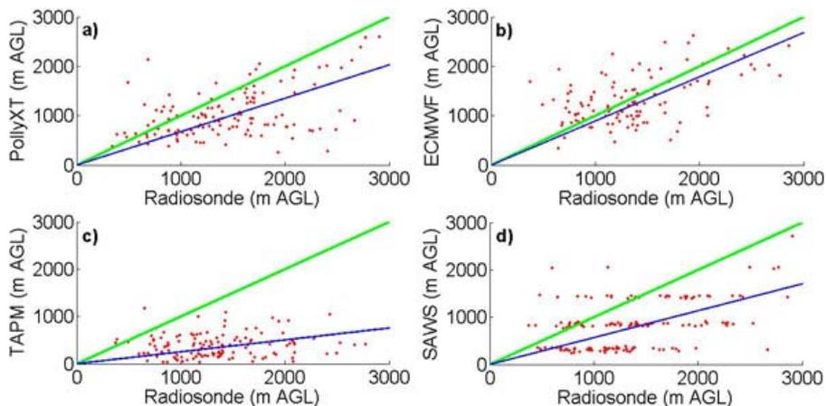
**Fig. 9.** Scatterplots for comparing Polly<sup>XT</sup> (a), the ECMWF (b), TAPM (c) and the SAWS model (d) to radiosonde observations in the comparison period. Blue and green lines mark linear fit to the data and 1 : 1 correlation, respectively.
