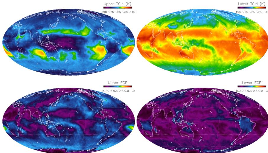
**Fig. 2.** The AIRS Standard L2 cloud top temperature  $T_C$  (upper row) and effective cloud fraction ECF (lower row) for the upper layer (left column) and lower layer (right column) for January 2007.
