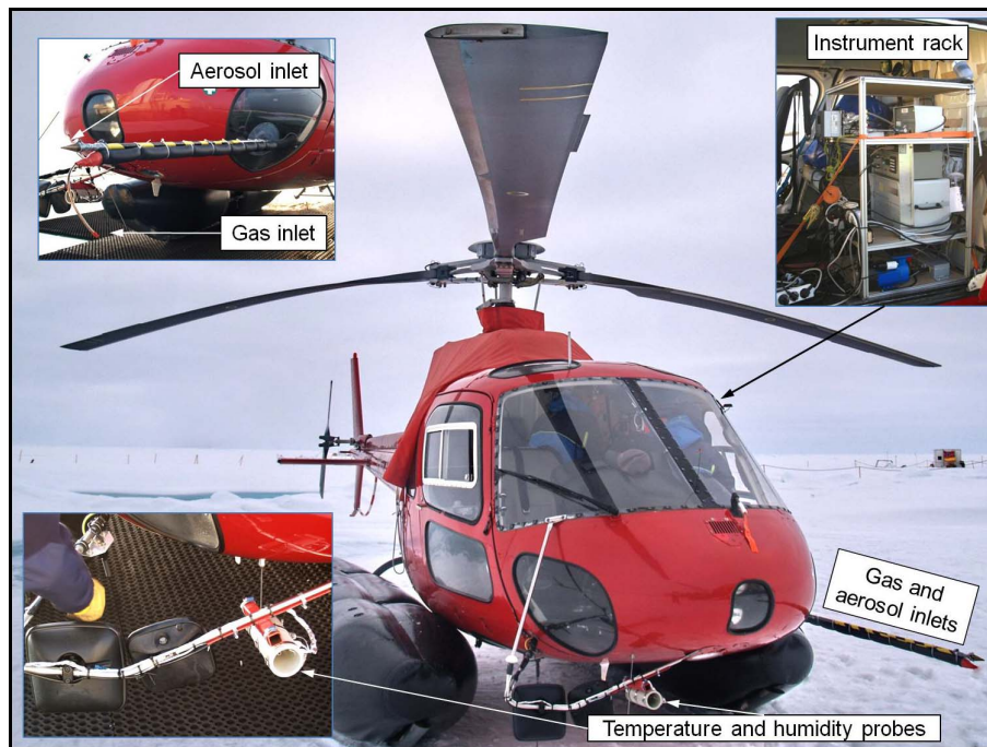
Fig. 10. Photograph of the helicopter that was used for vertical profiling, outlining some of the installations to sample meteorology, aerosol particles and trace gases.
