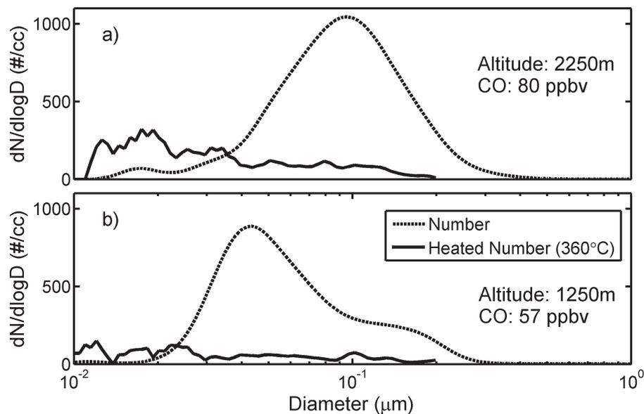
**Fig. 1.** Examples of DMA distributions in the FT from RF08 for a low CO layer and high CO layer before (dotted) and after heating to 360°C (solid).
