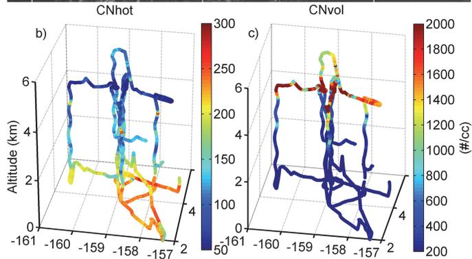
**Fig. 3.** OES image (a) showing cloud targeted for RF04 study. Flight path plots (bottom) color coded with CNhot (b) and CNvol (c). Horizontal legs to west, south and east flown in outflow layers at 4.3 km show marked depletions of CNhot and strong enhancement of CNvol relative to MBL.
